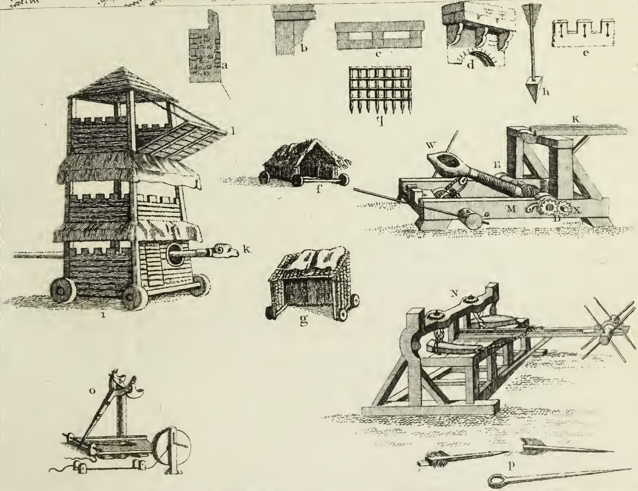
a. Section of the Wall of the Ballium. b. A Section. c. A Plan. d. A Perspective representation of a Machicolation. e. Crenellas. f. The Sow. g. The Gallus. h. A Dart called a Quarrel. i. A Movable Tower of three Stages. k. A battering ram. l. A Bridge to let down for storming. m. Catapult acting by counterpoise. n. Darts for the Ballista. o. Winch for bending it. p. Horse or Portcullis.
